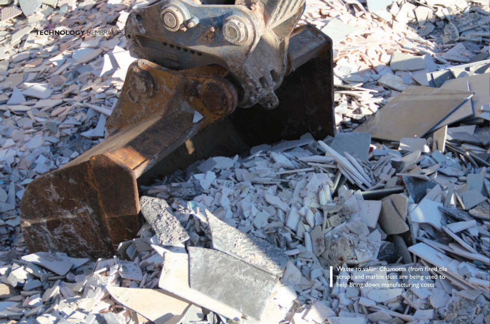
Waste to value: Chamotte (from fired tile scrap) and marble dust are being used to help bring down manufacturing costs
